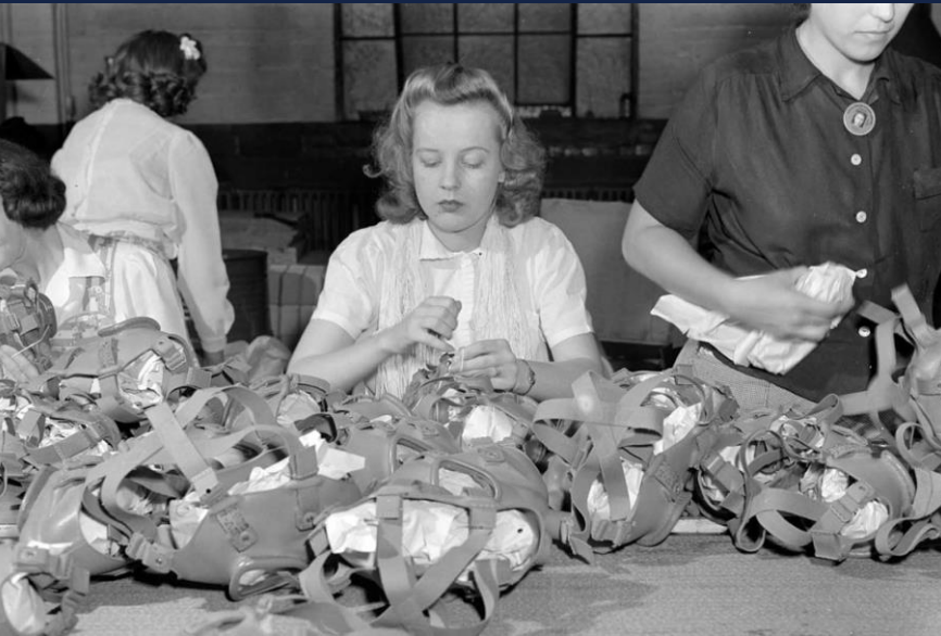
Women lacing head harnesses of gas masks in the Eureka Vacuum factory which has been converted to war production.
